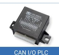
The all-round talent – the compact CAN I/O PLC with 14 inputs and outputs.
