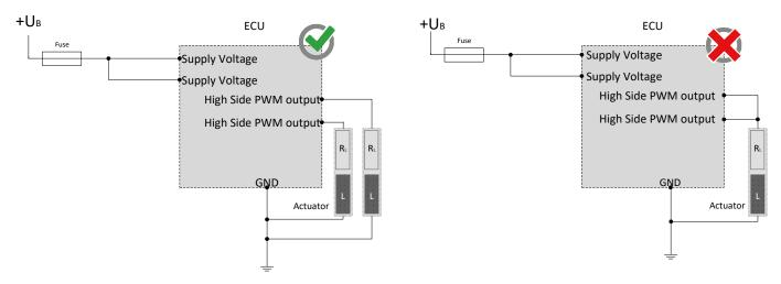
The pins (I/Os) can be used in combination and may not be switched externally against supply voltage.
